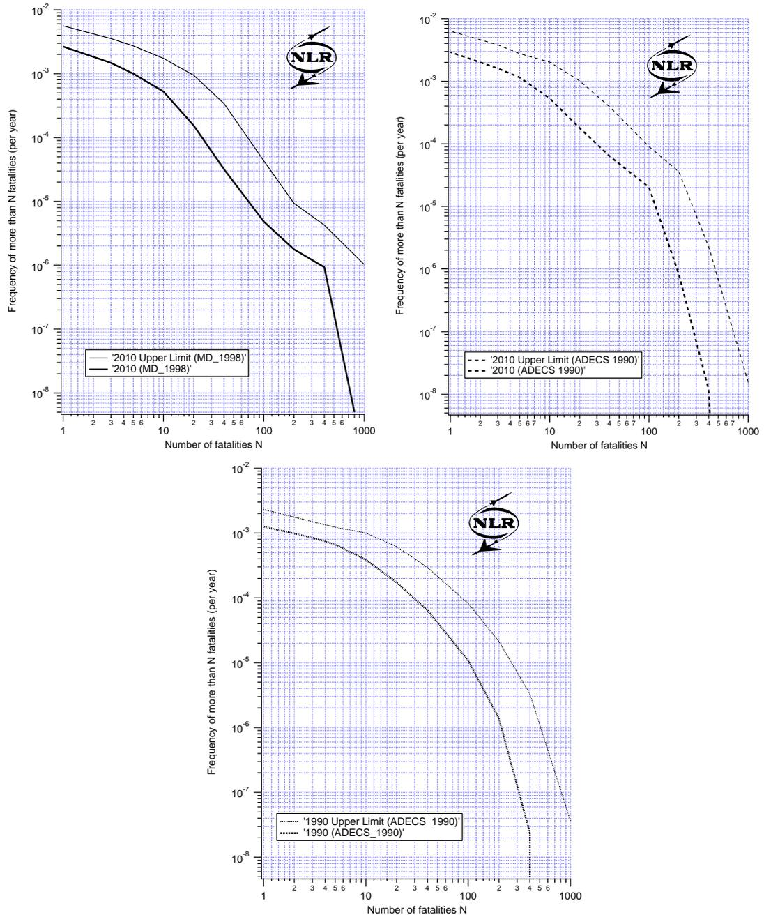
Figure 8-5: Estimates and upper limits of societal risk for: (top left) the S5P-2010 scenario evaluated with the MD 1998 population density file, (top right) the S5P-2010 scenario evaluated with the ADECS 1990 population density file, and (bottom) the S4S1-1990 scenario evaluated with the ADECS 1990 population density file.
